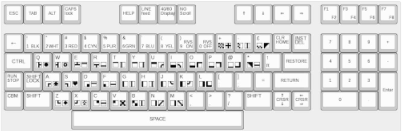
This mapping applies to the C128 emulator. It is for a large part identical with the respective C64 mapping, plus the added function- and extra keys.
