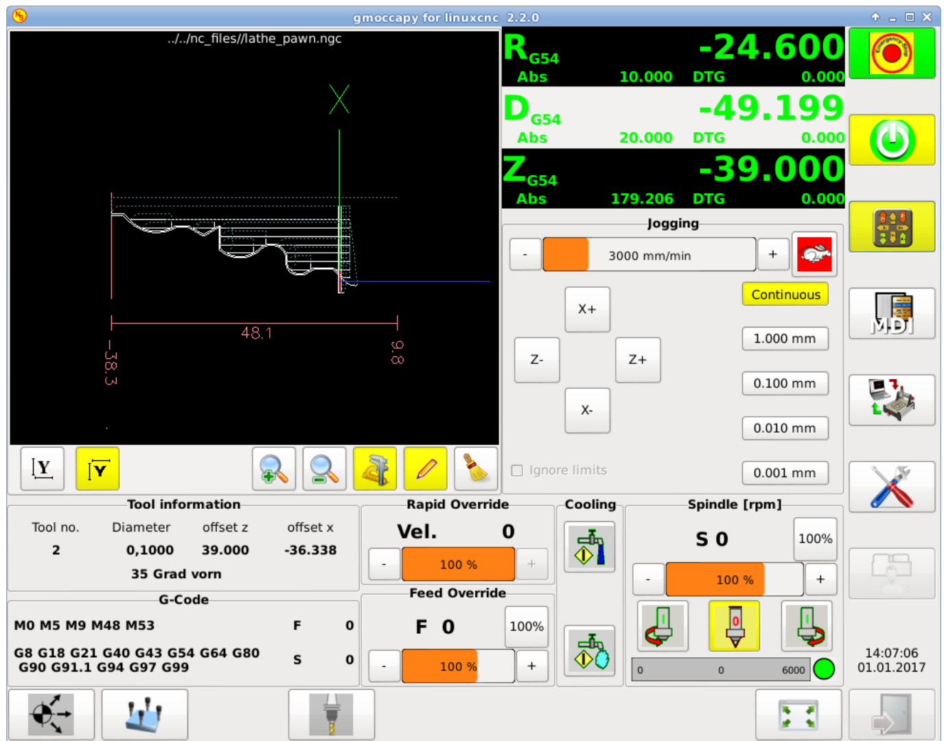
Figure 5.22: Back Tool Lathe
